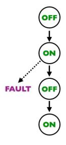
A testing tree can be drawn to represent a better, single test that would have detected this fault.
