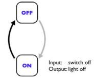
In the state of 'on' the system can be given another input, it can be switched off, and the system returns to the state of off. Again there is a measurable output, the light is switched off.
