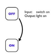
By giving the system an input, in this case switch it on, the system switches from the state of 'off' to the state of 'on'. In the process there is a measurable output, in this case the light comes on.
