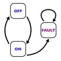
What actually happened is that during the second test the system developed a fault. This meant that it never entered the state of off, instead it entered a new state. This state has been called 'fault'.
